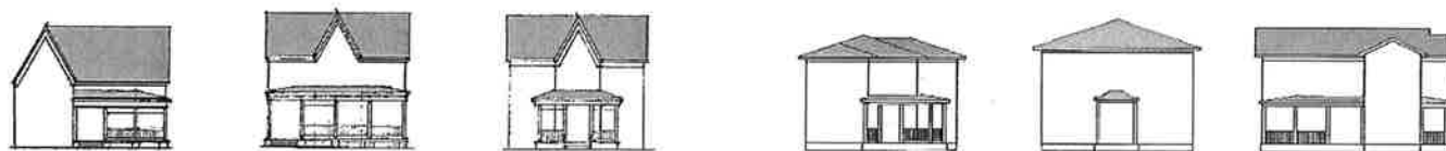
Carpenter Gothic Porch Locations
